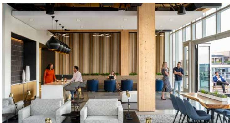
In Washington, DC's Capitol Riverfront district, zoning restricts building heights and undeveloped parcels are limited. Taking advantage of wood's lighter weight, 80 M Street's 9,000-square-metre rehabilitation overbuild introduces two floors and a rooftop level to a seven-storey steel and concrete building completed in 2001, adding leasable area without needing to reinforce the structure below.
